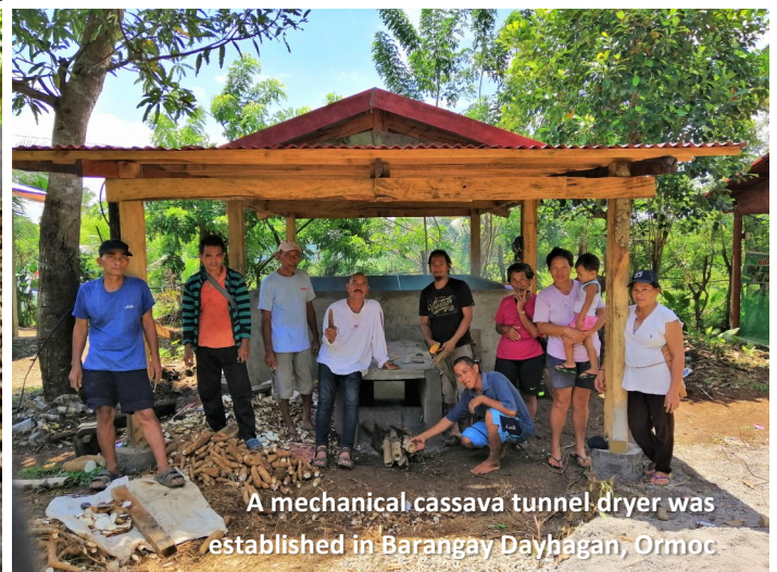
The heat comes from fire that is being evenly distributed inside the dryer by a mechanical blower
